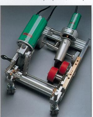
the past. The BAS concept is quite ingenious: a set of propelled silicone wheels is incorporated to a Leister Variant 4R5. These wheels keep the sheets under controlled pressure before hot air welding, resulting in a perfectly flat seam. A BAS modified machine is part of the equipment used at the Rubberfuse Mappano,(1) Training Centre.
